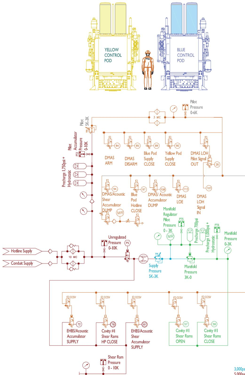
This schematic shows the typical hydraulic controls in one of the two redundant pods used to control only one set of shear rams.
