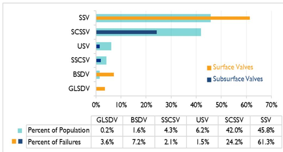
**NOTE:** Includes 194 total failures. Excludes 20 failures of subsurface safety valves identified in OGOR-A data where it could not be confirmed whether they were SCSSVs or SSCSVs.
