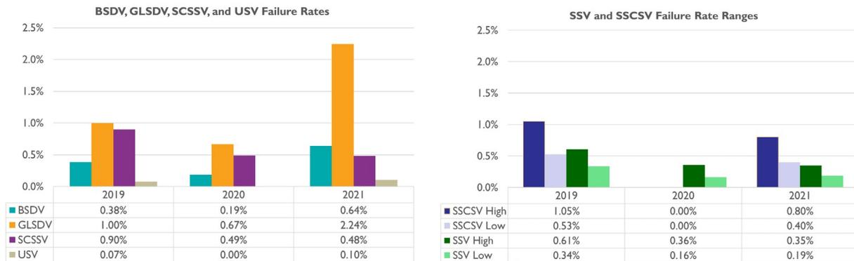
**NOTE:** 2019 includes 329 total failures and excludes 22 failures of unknown SSSV type. 2020 includes 159 failures and excludes 13 failures of unknown SSSV type. 2021 includes 194 total failures. Excludes 20 failures of subsurface safety valves identified in OGOR-A data where it could not be confirmed whether they were SCSSVs or SSCSVs. The right-hand plot reflects a failure rate range for SSCSVs and SSVs due to variability in testing frequency, described further in Appendix E.
