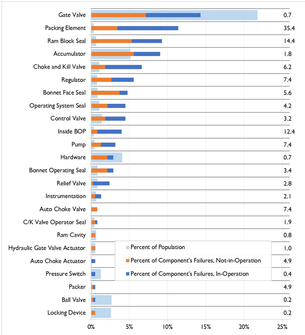
**NOTE:** Components with 0.5 percent or less of failures are excluded and total 6.7 percent of all surface system failures. Piping/tubing (1.3 percent of failures) is not represented in the table as it does not have an estimated population average. Failure ratio, shown in righthand column, represents the component's percent of failures divided by that component's percent of the population.
