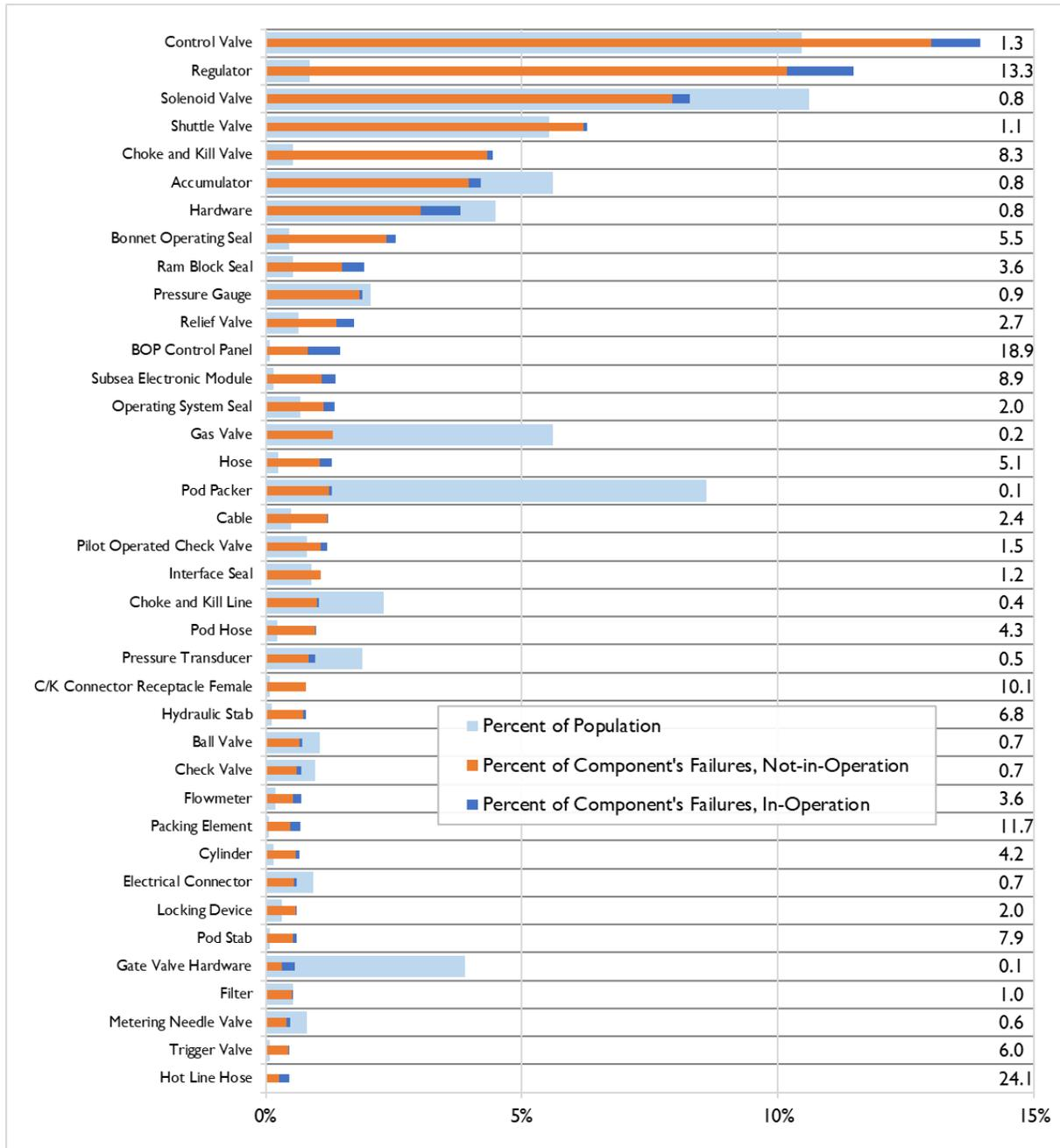
**NOTE:** Components with 0.5 percent or less of failures are excluded and total 10.4 percent of all subsea system failures. Piping/Tubing (5.1 percent of failures) and Studs and Nuts (0.1 percent of failures) are not represented in the table as they do not have an estimated population average. Failure ratio, shown in righthand column, represents the component's percent of failures divided by that component's percent of the population.
