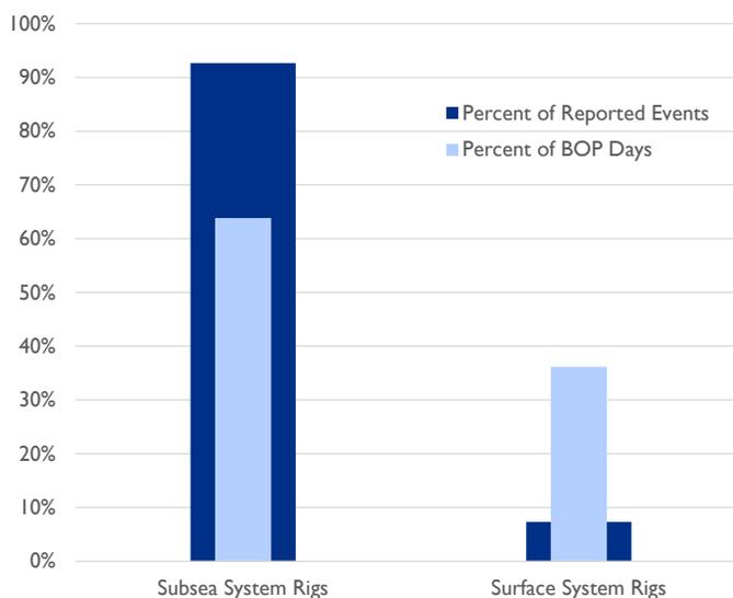
**NOTE:** Subsea system rigs represented include drillships, semisubmersibles, and dynamically positioned (DP) semisubmersibles. Surface system rigs represented primarily include platform rigs and jackups.
